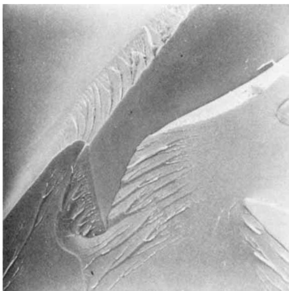
Fig. 4. Fracture face of a 107-hr water-boil-treated styrene-crosslinked polyester ( $\times 480$ ).
